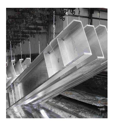
At Rigel Exports, we specialize in providing high-quality hot-dip galvanizing services to protect steel and iron components from corrosion. Our state-of-the-art facility and experienced team ensure that your products receive the best treatment for enhanced durability and longevity. Whether you're working on large infrastructure projects or small-scale industrial applications, our galvanizing process guarantees superior protection.
